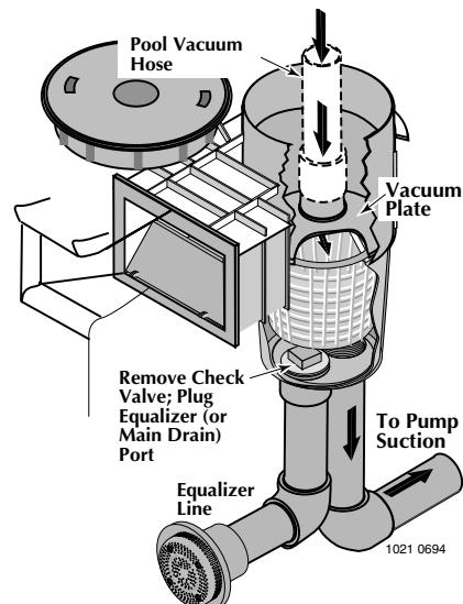
Figure 4: To vacuum pool, remove
