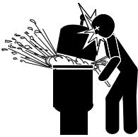
THIS FILTER OPERATES UNDER HIGH PRESSURE. WHEN ANY PART OF THE CIRCULATING SYSTEM (e.g., CLAMP, PUMP, FILTER, VALVES, ETC.) IS SERVICED, AIR CAN ENTER THE SYSTEM AND BECOME PRESSURIZED. PRESSURIZED AIR CAN CAUSE THE LID TO BE BLOWN OFF WHICH CAN RESULT IN SEVERE INJURY, DEATH, OR PROPERTY DAMAGE. TO AVOID THIS POTENTIAL HAZARD, FOLLOW THESE INSTRUCTIONS.
