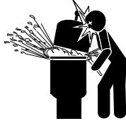
CE FILTRE EST SOUS HAUTE PRESSION. LORS DE LA MAINTENANCE DE N'IMPORTE QUEL COMPOSANT DU SYSTÈME DE CIRCULATION (TEL QUE COLLIER DE SERRAGE, POMPE, FILTRE, SOUPAPES, ETC.), ON RISQUE D'INTROUVER DE L'AIR DANS LE SYSTÈME ET DE LE COMPRIMER. OR L'AIR COMPRIMÉ PEUT FAIRE SAUTER LE COUVERCLE ET ENTRAÎNER PAR LÀ BLESSURES GRAVES, DÉCÈS OU DÉGÂTS MATÉRIELS. POUR PRÉVENIR CE DANGER, PRIÈRE D'OBSERVER LES DIRECTIVES INDIQUÉES CI-DESSOUS.
