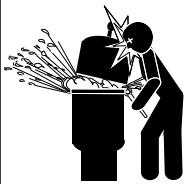
**CE FILTRE EST SOUS HAUTE PRESSION. LORS DE LA MAINTENANCE DE N'IMPORTE QUEL COMPOSANT DU SYSTÈME DE CIRCULATION (TEL QUE COLLIER DE SERRAGE, POMPE, FILTRE, SOUPAPES, ETC.), ON RISQUE D'INTRODUIRE DE L'AIR DANS LE SYSTÈME ET DE LE COMPRIMER. OR L'AIR COMPRIMÉ PEUT FAIRE SAUTER LE COUVERCLE ET ENTRAÎNER PAR LÀ BLESSURES GRAVES, DÉCÈS OU DÉGÂTS MATÉRIELS. POUR PRÉVENIR CE DANGER, PRIÈRE D'OBSERVER LES DIRECTIVES INDIQUÉES CI-DESSOUS.**
