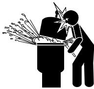
THIS FILTER OPERATES UNDER HIGH PRESSURE. WHEN ANY PART OF THE CIRCULATING SYSTEM (e.g., CLAMP, PUMP, FILTER, VALVES, ETC.) IS SERVICED, AIR CAN ENTER THE SYSTEM AND BECOME PRESSURIZED. PRESSURIZED AIR CAN CAUSE THE LID TO BE BLOWN OFF WHICH CAN RESULT IN SEVERE INJURY, DEATH, OR PROPERTY DAMAGE. TO AVOID THIS POTENTIAL HAZARD, FOLLOW THESE INSTRUCTIONS.
