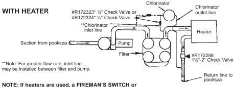
equivalent must be installed to prevent possible damage and improper operation of CHECK VALVE and other equipment subject to heat damage.
