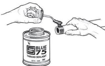
**STEP 2** **Assemble Joint by Hand** - Threaded pipe and valves must be initially assembled "finger tight" (just enough to fully engage thread clearance).
