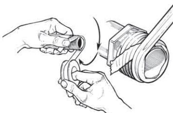
**STEP 1** **Apply Joint Sealant** - Threaded connections require application of a quality grade thread sealant to seal and lubricate joint assembly. Sealant must be applied to male pipe threads.
