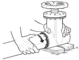
**STEP 8** **Remove Excess Cement**
