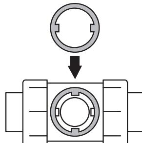
2. For Lock-Open Only (prevents valve from being locked in the closed position): cement lock ring on body stem tower with lugs perpendicular to valve and pipe line.
