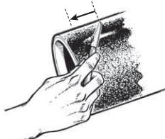
Check the penetration and softening by scraping the primed surfaces. A few thousandths of the semi-fluid surface should easily be removed.
