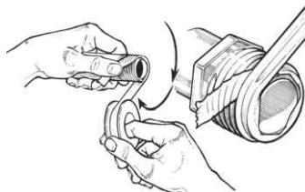
**STEP 1** Apply Joint Sealant -
