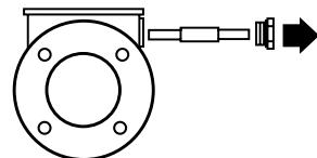
**Step 3:** Insert one (1) Shaft Cup Seal with flat side OUT into recess of valve body until seated. Insert Extended Shaft through Cup Seal into valve and disc with stem flat aligned with flat on disc.
