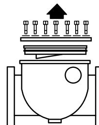
**Step 2:** Remove Stem Cap Nut from shaft end on side of valve and pull shaft from disc and valve.
