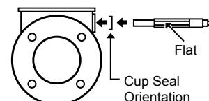
**Step 4:** Install one (1) Shaft Cup Seal with flat side IN over shaft end until seated. Note: both Cup Seals must be oriented with flat side facing each other. Install new Stem Nut. Tighten Stem Nut snug, but do not over tighten. Note: O-ring is NOT TO BE USED on new Shaft Nut.
