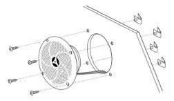
Using the drilling template supplied with the unit select the most appropriate location on wall for the speakers. For flush mounting a depth of at least  $2\,3/16$ " (55 mm) will be required. Mark the location and with a hole saw make a cutout of  $4\,3/8$ " (111 mm) in diameter. As indicated on the template, drill the four (4) holes of 3/16" (5 mm) in diameter. Insert the speaker in place, use 4- M30 screws to fix the speakers (supplied in package to fix).
