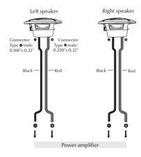
Connect the speaker terminals to the Speaker In terminals on the amplifier.
