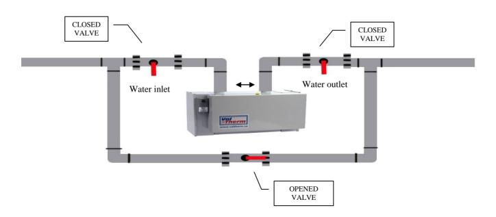
It is recommended to isolate your water heater on the water by-pass when you do your shok treatment at the opening of your pool not to damage the component.
