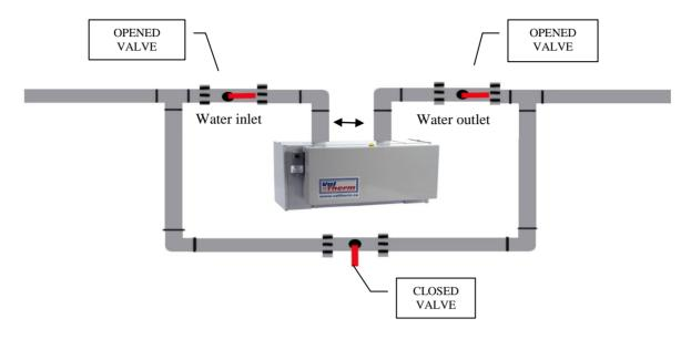
It is recommended to install a by-pass on the plumbing of the water heater.
