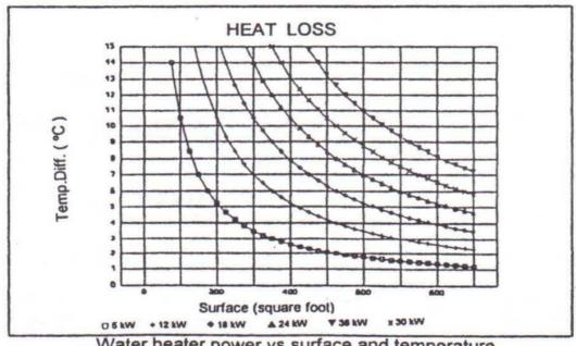
Water heater power vs surface and temperature
