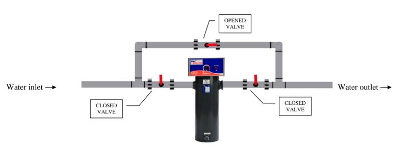
It is recommended to isolate your water heater on the water by pass when you do your shock treatment at the opening of you pool not to damage the component.
