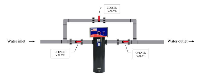
It is recommended to install a by-pass on the plumbing of the water heater.
