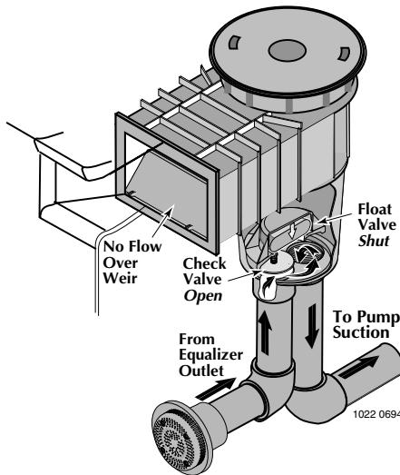
Figure 3: Equalizer operation: Float
