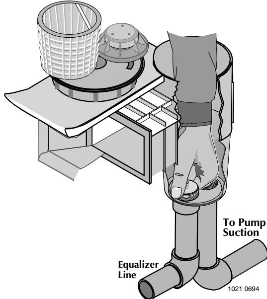
Figure 1: Check valve installation. Tighten finger-tight only.
