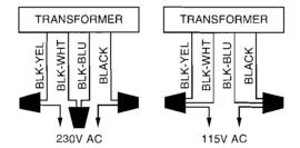
The high voltage wiring section is located behind the service panel in the lower right side compartment of the Solar Control. Holes are provided on bottom of enclosure for conduit mounting. The Solar Control can be connected either to 115VAC or 230VAC. The Solar Control should be wired so that it gets continuous power (connect to Line-Side of Time Clock or directly to sub-panel).
