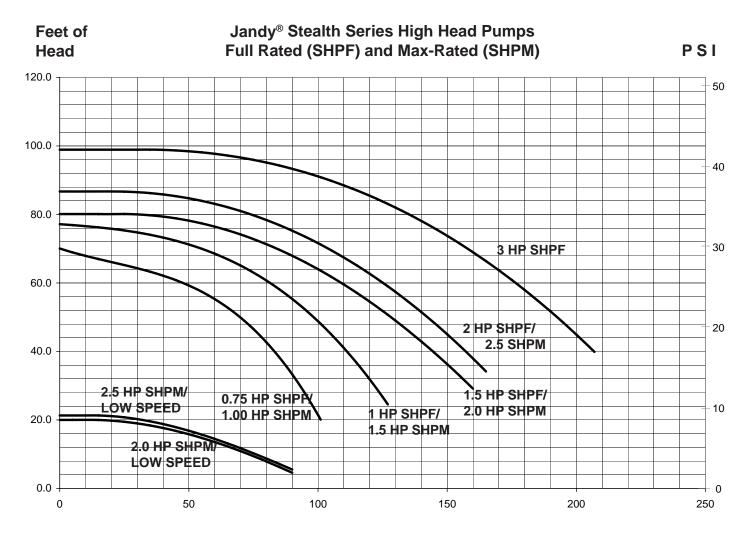
Flow Rate (GPM)
