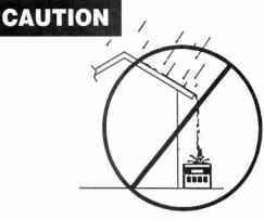
DO NOT INSTALL MINIMAX HEATERS UNDER ANY ROOF OVERHANGS NOT HAVING RAIN GUTTERS, EXCESS WATER MAY FLOOD HEATER. DOES NOT APPLY TO OUTDOOR POWERMAX VERSIONS.
