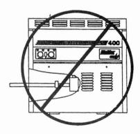
DO NOT PLACE GAS SUPPLY LINE UNION COUPLING INSIDE OF HEATER JACKET.
