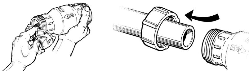
**STEP 4** Place Rubber Gasket over pipe end .
