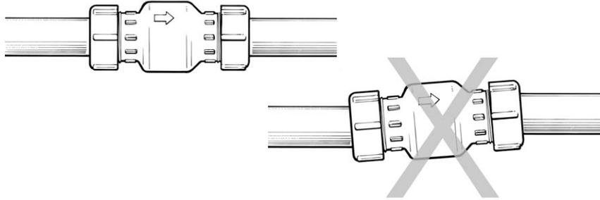
**STEP 7** Use SPEARS® Compression Nut Wrench or commercially available Strap Wrench only. **Do not use conventional pipe wrenches that can damage plastic materials.** Tighten Nuts Hand Tight plus approximately ¼ to ½ turns. Average torque should be approximately 25 ft-lbs on valve sizes ½ to 2 inches.
