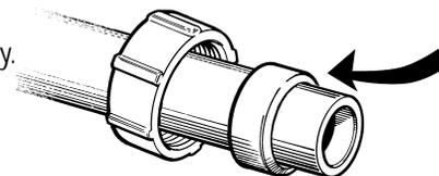
**STEP 5** Join pipe and gasket to valve body by firmly inserting both into socket. Slide Union Nut over gasket to engage threads. Hand tighten only.
