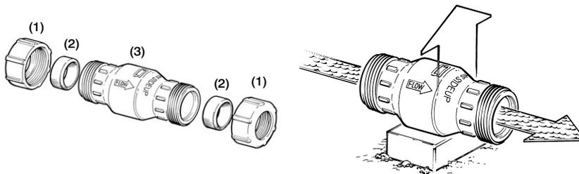
**STEP 3** Wipe away all loose dirt & moisture from the pipes & components with a clean dry cloth. Slide Union Nuts (1) over pipe ends, being sure that the Union Nut threads will be facing the Valve body.
