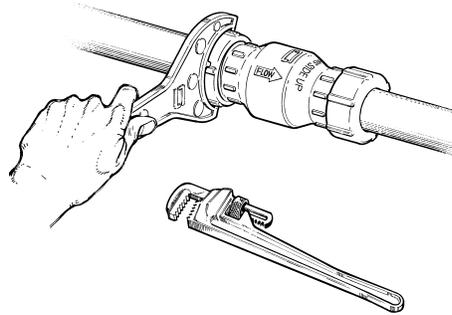
**STEP 8** Pressure test system only after all joints have been properly tightened.
