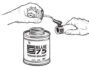
**STEP 1 Apply Joint Sealant** - Threaded connections require application of a quality grade thread sealant to seal and lubricate the joint assembly. Sealants must only be applied to male pipe threads.
