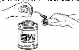
**STEP 1** - Apply Joint Sealant
