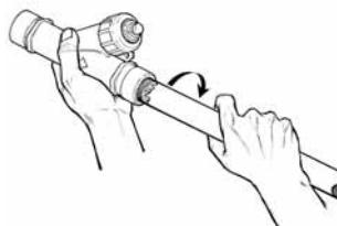
**STEP 2** Assemble Joint - 1 to 2 turns beyond "FINGER TIGHT" are generally all that is required to make a sound plastic threaded connection.
