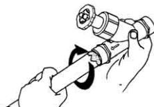
Unnecessary OVER TIGHTENING will cause damage to both pipe and Y-Pattern valve threads.
