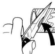
Check the penetration and softening by scraping the primed surfaces. A few thousandths of the semi-fluid surface should easily be removed.
