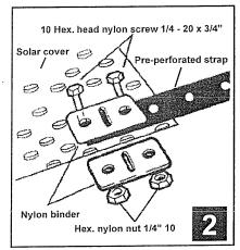
When you install the straps to the solar cover, they must be in equal distance one from the other. The straps length must be adjust in function of the shape of the pool.
