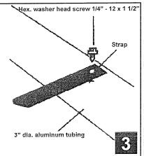
You must drill holes in aluminum tubing to fix straps which are already attached to solar cover.
