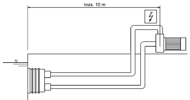
Suctionpipe with 2 bends Pressurepipe with 3 bends
