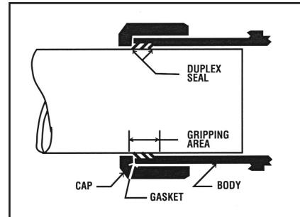
**Duplex Seal** – Compressive action of thread cap creates high concentrated pressure at two points illustrated. Since cap and body are recessed for compression sealing gasket, no fluid can enter thread cavity of cap.
