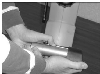
3. Push the Front Molded Feet onto the Front Support Leg.
