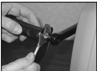
6. Insert the threads of the Right Pedal into the Right Pedal Crank, and with the wrench, turn it counter clockwise until it is snug. Repeat this process for the Left Pedal.
