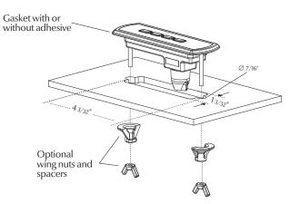
To install the in.kl $00^{\text{in}}$ , determine the mounting location and cut out a rectangular shape opening of  $43/32^{\text{r}}$  by  $13/32^{\text{r}}$  (see illustration).
