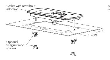
To install the in.k600<sup>™</sup> low profile, determine the mounting location and cut out a rectangular shape opening of 7.250" by 3.750" (see illustration).
